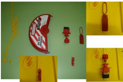
Various Types of Isolators
