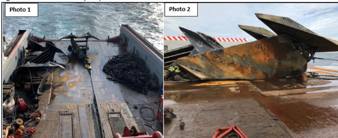
Photo 1: Anchor recovered to deck. Photo 2: Banff Anchor 02 Stevpris 50 Te.
