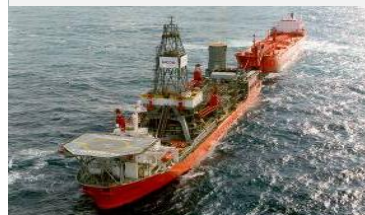
Petrojarl I FPSO
